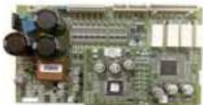
Escalator Extension Board
