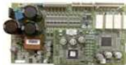
Escalator Extension Board
