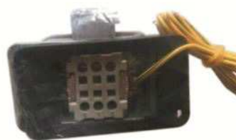
Control Cabinet Plug
